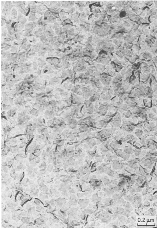
Figure 2 Transmission electron micrograph of a polyethylene coat (HB 301) after coating on to the polypropylene substrate, but prior to any thermal treatment.
